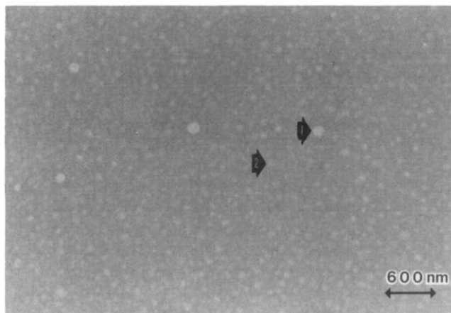
Figure 12 Transmission electron micrograph of a solution cast film of 53% chlorinated PB. Region 1 = holes. Region 2 = partial holes or unchlorinated PB domains
